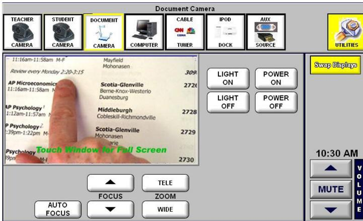
Zoom, Focus and Lamp adjustments can be made either on the touch screen or directly on the document camera control pad.
