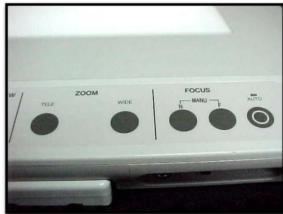
**Focus** Allows you to manually fine tune the focus of the image displayed. (It is also possible to adjust focus by turning the lens by hand.)
