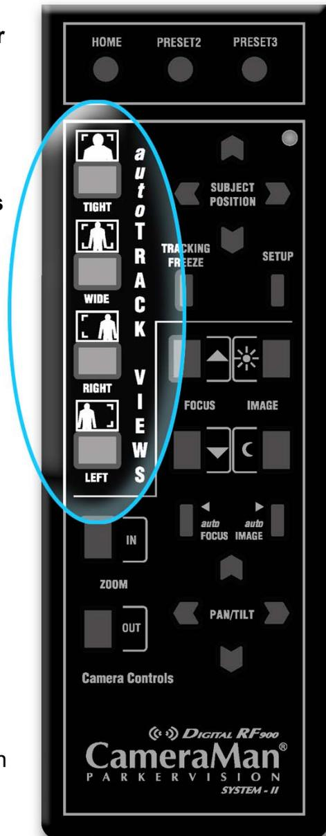
The keypad will not function with weak or dead batteries. It does not come equipped with rechargeable batteries. Check inside the rear of your keypad for battery type. Although most keypads use two (2) AA batteries, some use 9-volt batteries.
