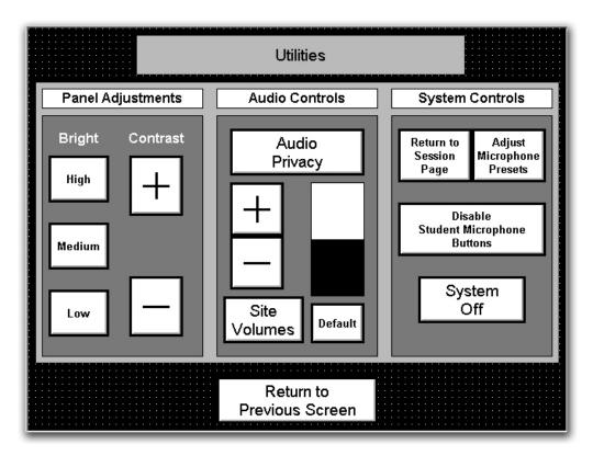
**<u>Panel Adjustments</u>** allow you to control the brightness and contrast of the touch screen display.
