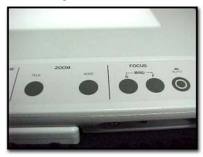
**Focus** Allows you to manually fine tune the focus of the image displayed. (It is also possible to adjust focus by turning the lens by hand.)
