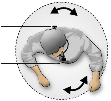
When the teacher turns around to point to a map, for example, the back sensor continues to receive the infrared tracking signal from the camera and the camera will continue to automatically track the teacher's movement.
