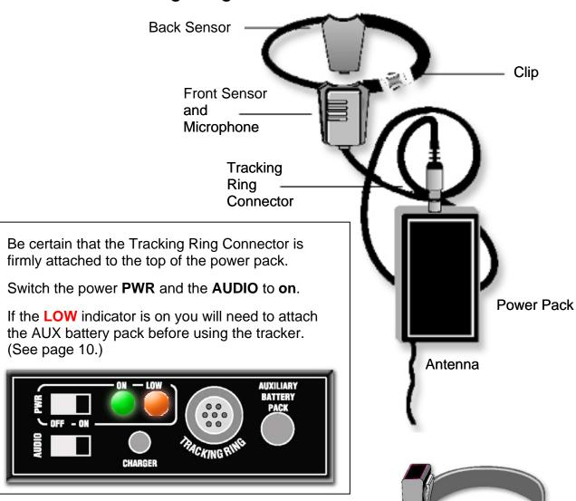
Attach the tracking ring power pack to your clothing or the nylon power pack belt.
