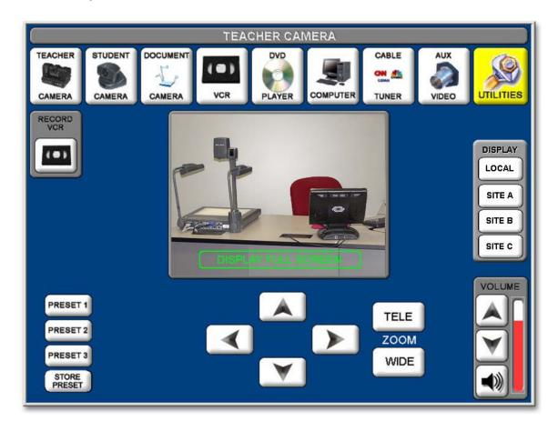
Touching the green area in the center box that reads "DISPLAY FULL SCREEN" will fill the touch screen with the video representation of your transmitted signal. To return the screen to normal control function, touch the full video image anywhere on the screen.
