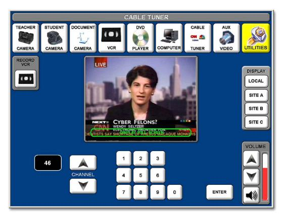
The channel number is displayed in the oval to the left of the channel up/down control.
