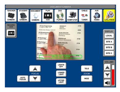
Zoom, Focus and Lamp adjustments can be made either on the touch screen or directly on the document camera control pad.
