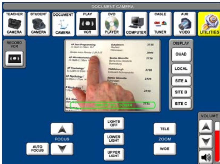
Zoom, Focus and Lamp adjustments can be made either on the touch screen or directly on the document camera control pad.
