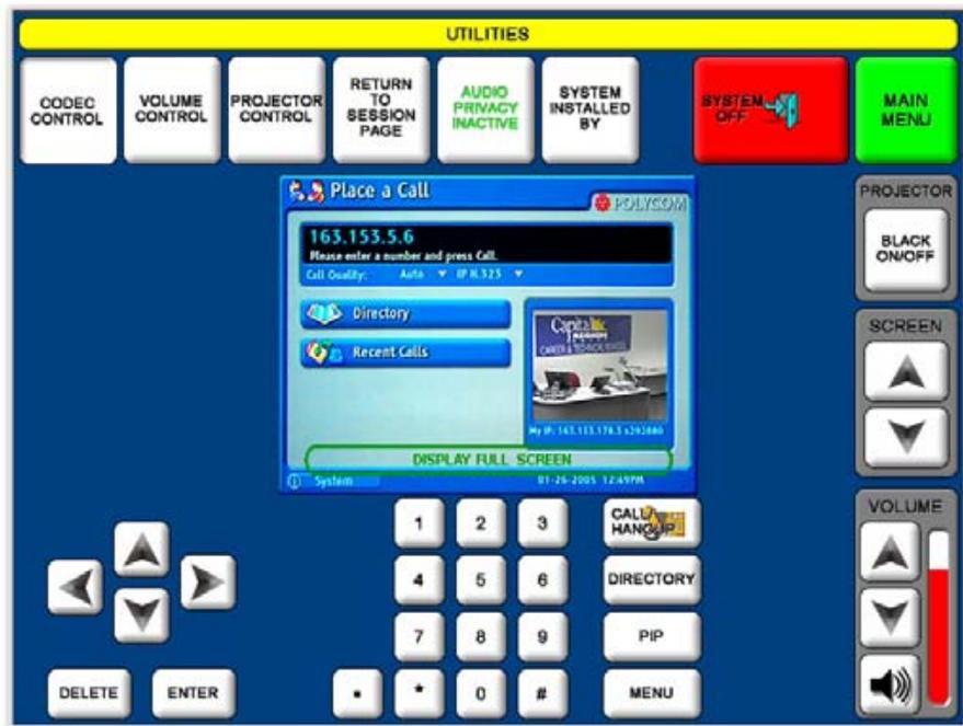
Use the keypad in the lower left of the screen to navigate the Polycom call menu. Use the number pad to enter the IP address that you wish to connect to.
