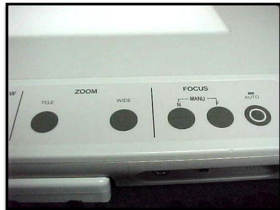
**Focus** Allows you to manually fine tune the focus of the image displayed.
