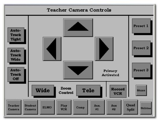
There are three types of camera presets that can be established, Teacher Camera Presets, Student Camera Presets and Student Microphone Presets. The procedure is similar in each case.
