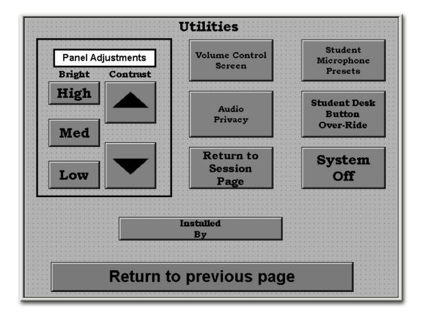
**<u>Panel Adjustments</u>** allow you to control the brightness and contrast of the touch screen display.
