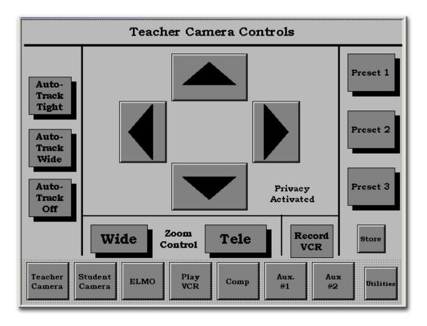
The buttons on the bottom of the screen are similar to a tool bar and appear on most screens selected.
