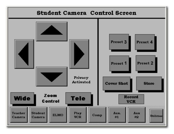
The student camera presets are established so the teacher or the aide can select preset student camera views using the Student Camera Control screen on the touch panel.
