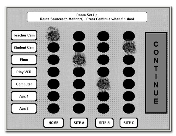
The seven buttons at the left of the screen correspond to the video source options. The four buttons at the bottom correspond to the four monitors in the front and rear of the room.
