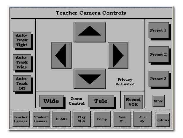
The buttons on the bottom of the screen are similar to a tool bar and appear on most screens selected.
