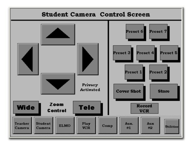
The student camera presets are established so the teacher or the aide can select preset student camera views using the Student Camera Control screen on the touch panel.
