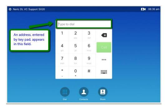
When the **Dial** button is pressed, the above screen will appear. Using the key pad, you can enter a numerical address such as an IP address (ex. 163.153.231.58) or an E164 number (ex. 518862530158).
