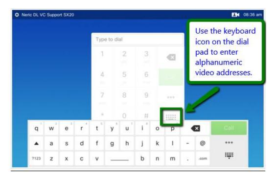
When a full QWERTY keyboard is needed to enter an endpoint address to which you are trying to connect, select the keyboard icon button on the lower right corner of the Dial pad. The above keyboard pop-up will appear. The full keyboard is usually needed for alpha-numeric addresses as in:
